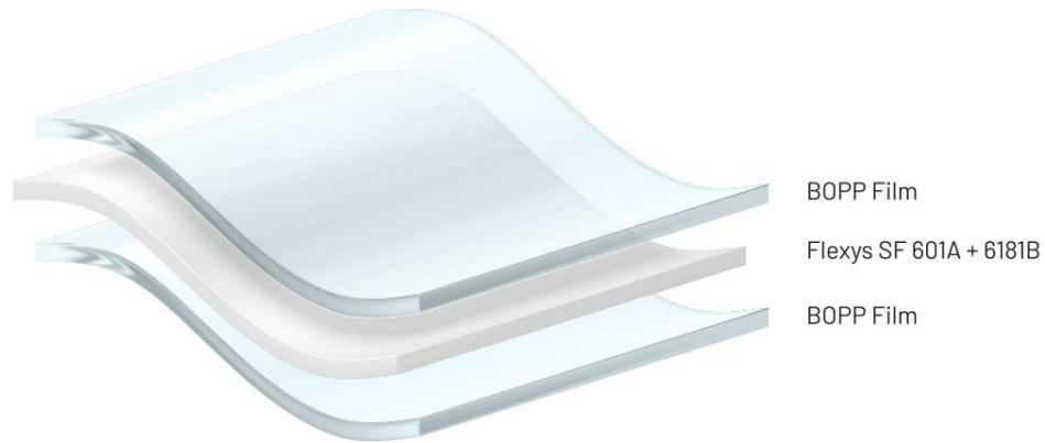
Figure 1. 'Frimpeks Flexys SF 601A/6181B' technology by Frimpeks used as laminating adhesive.
