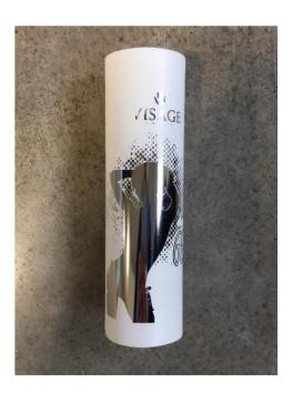
Figure 1: Tested cold transfer 'InLine Foiling' technology by Leonhard Kurz.
