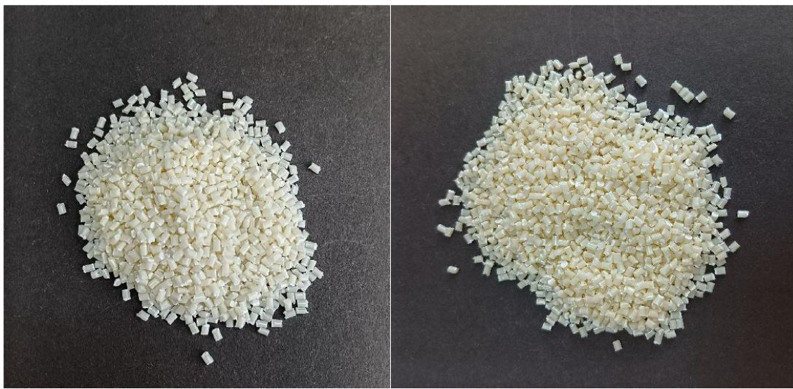
Figure 1. Extruded “ELIX ABS HH 3110” resin by Elix Polymers. 1 st and 2 nd extrusion (left to right) performed by Proplast.
