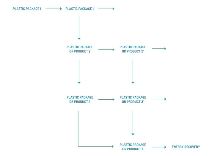
Fig. 2 Cascade open-loop recycling
