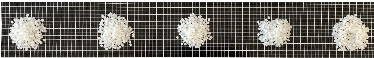
FIGURE 4. PELLETS PRODUCED AFTER EXTRUSION (HDPE) (A.0, A1.25, A1.50, A2.25, A2.50 FROM LEFT TO RIGHT)
