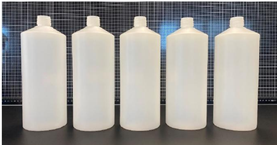
FIGURE 8. BOTTLES PRODUCED BY BLOW MOULDING (HDPE) (B.0, B1.25, B1.50, B2.25 AND B2.50 FROM LEFT TO RIGHT)
