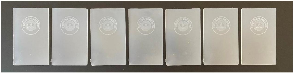
FIGURE 6. INJECTED PLAQUES PRODUCED BY INJECTION MOULDING (PP) (A.0, A4.25, A4.50, A5.25, A5.50, A6.25, A6.50 FROM LEFT TO RIGHT)
