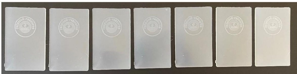
FIGURE 5. INJECTED PLAQUES PRODUCED BY INJECTION MOULDING (PP) (A.0, A1.25, A1.50, A2.25, A2.50, A3.25, A3.50 FROM LEFT TO RIGHT)
