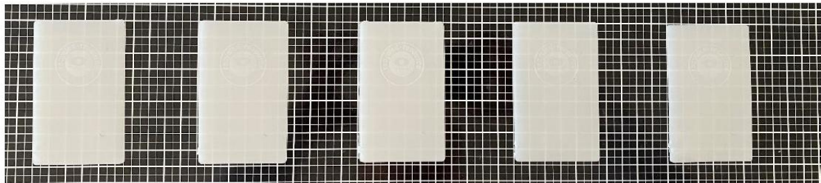
FIGURE 7. INJECTED PLAQUES PRODUCED BY INJECTION MOULDING (HDPE) (A.0, A1.25, A1.50, A2.25, A2.50 FROM LEFT TO RIGHT)
