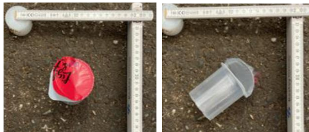
Figure 2. PS yogurt pot with PS banderole and PET lid (Sample 2). Please note that samples 2 had transparent and non-printed OPS banderole.
