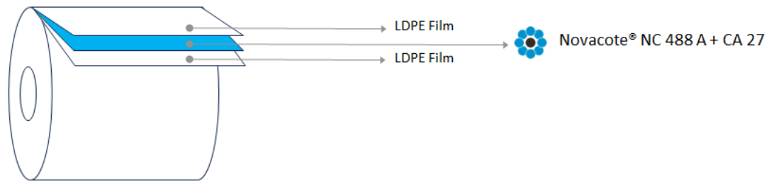
Figure 1. 'Novacote® NC 488 A + CA 27' technology by C.O.I.M. used as laminating adhesive
