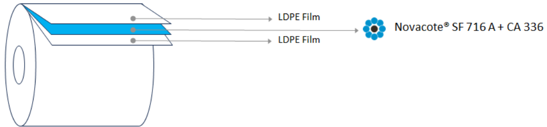
Figure 1. 'Novacote® SF 716 A + CA 336' technology by C.O.I.M. used as laminating adhesive
