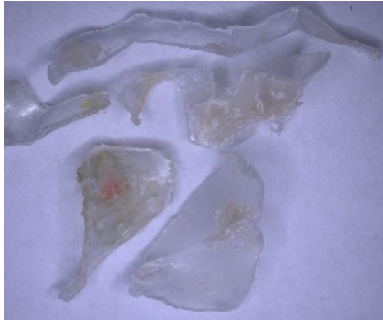
Glue residues on flakes
