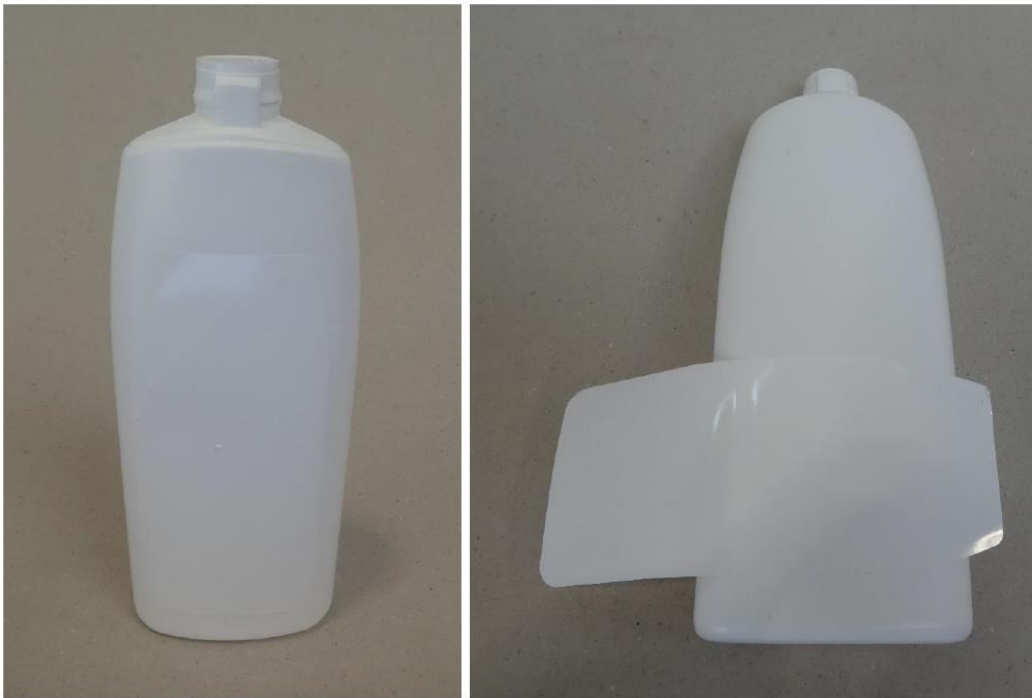
Figure 1. 'PP60 TOP WHITE – Acrylic Adhesive, Film Thickness \leq 60 \mu\text{m} ' by Avery Dennison without cap and unprinted
