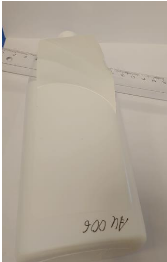
Figure 1. 'GLOBAL MDO TOP WHITE – Acrylic Adhesive, Film Thickness \leq 50\mu\text{m} ' by Avery Dennison without cap and unprinted
