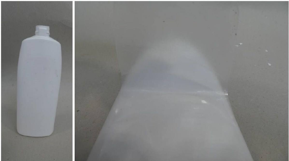
Figure 1. 'PE TOP CLEAR - Acrylic Adhesive' by Avery Dennison without cap and unprinted
