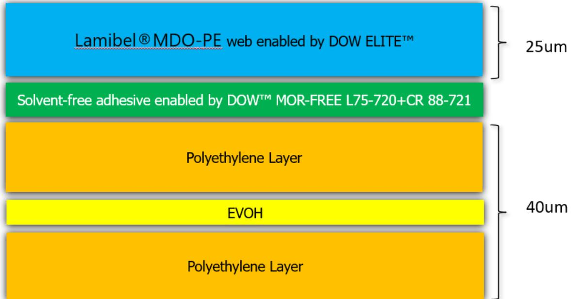
Figure 1 'Lamibel® MDO-PE Laminated HB' technology by Walki Plasbel.
