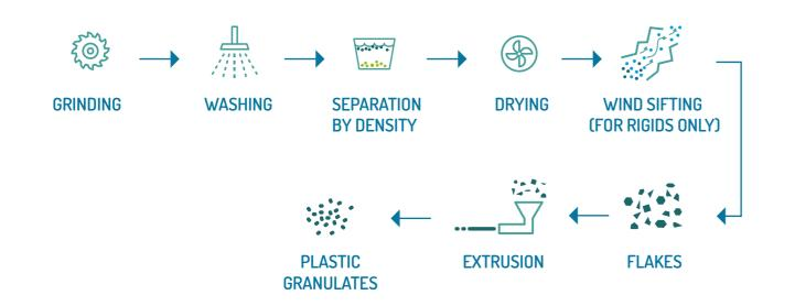
GRINDING Packaging is shredded to obtain plastic flakes.
