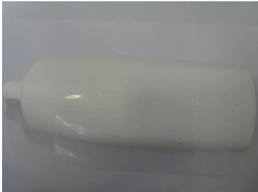
Figure 1. PP top clear with S692N acrylic adhesive, Film Thickness \leq 60 \mu\text{m} by Avery Dennison without cap and unprinted.
