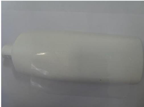
Figure 1. PP top clear with Acrylic adhesive, Film Thickness \leq 60 \mu\text{m} by Avery Dennison without cap and unprinted.
