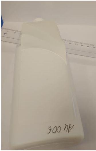
Figure 1. Global MDO top white with S7000 acrylic adhesive, Film Thickness \leq 50 \mu\text{m} by Avery Dennison without cap and unprinted.
