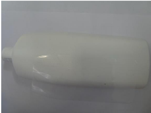
Figure 1. PE top white with S692N acrylic adhesive by Avery Dennison without cap and unprinted.
