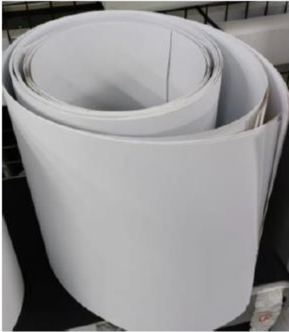
Figure 1. PS/Tie layer/EVOH/Tie layer/PS, provided by Cobelplast.
