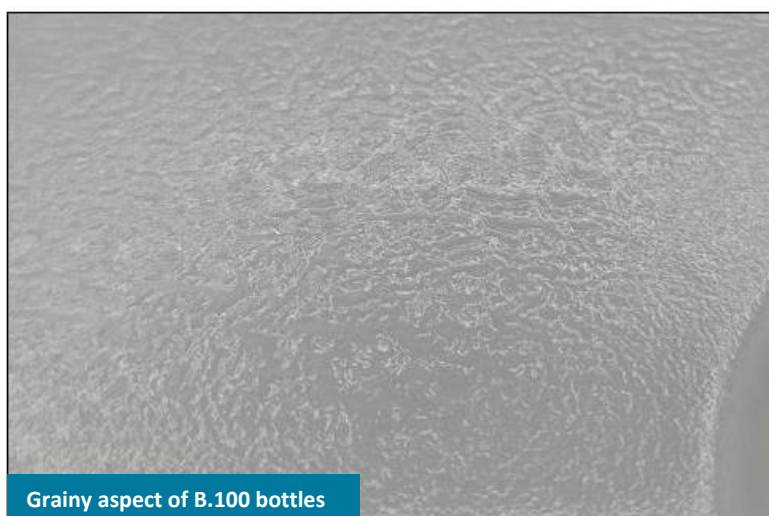
Figure 2: Parison defects during blow moulding process for samples containing foamed liners
