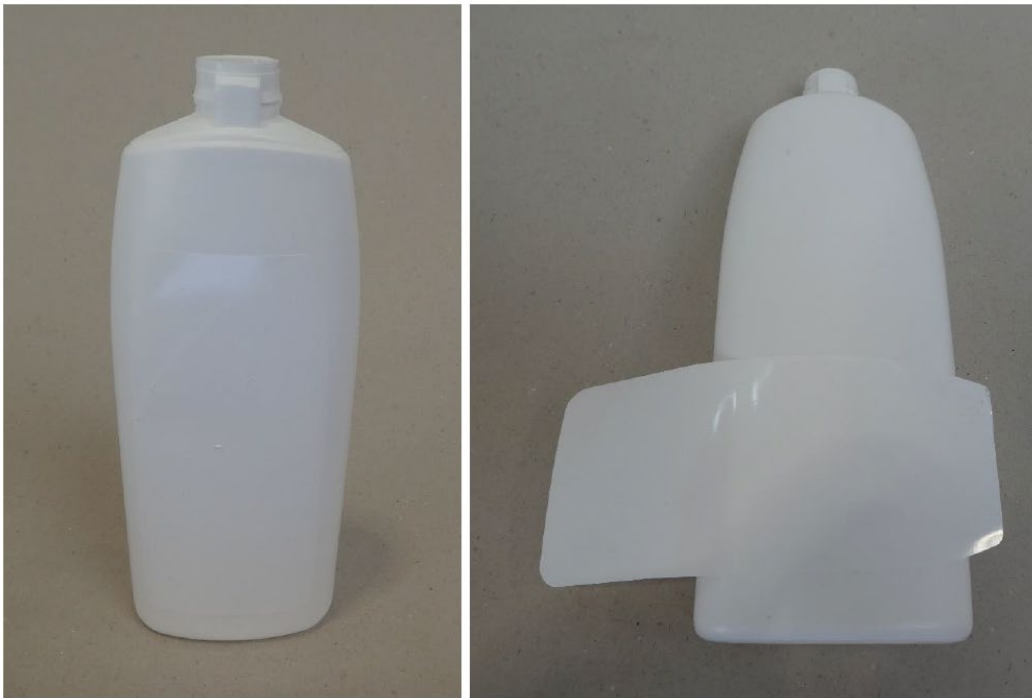
PP60 TOP WHITE – Acrylic Adhesive, Film Thickness \leq 60\mu\text{m} by Avery Dennison without cap and unprinted
