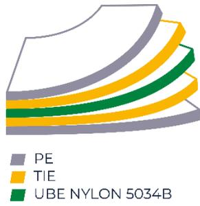
*Figure 1 PERFORMANCE PA SC15 technology by UBE*
